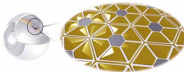
*The RetinaSensor is illustrated as subretinal implant in a human eye. It contains highly sensitive photodetectors for capturing incoming light. The resulting electrical signals from the photodetectors are sent to the petal-shaped electrodes for retinal stimulation with a novel biomimetic stimulation paradigm.*
