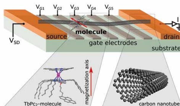
Single-molecule magnet grafted on a suspended CNT.  $V_{SD}$ : applied bias between source and drain electrode,  $V_{G1}, \dots, V_{G5}$ : bias applied to capacitively coupled gate electrodes 1 to 5 to drive mechanical oscillations in the CNT,  $I$ : measured current through the CNT
