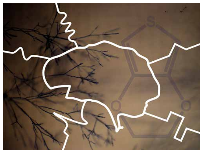
The research project aims to realize neuromorphic functions based on organic semiconductors. For example, fiber structures made of poly-3,4-ethylenedioxythiophene, can be used for this purpose. The structural formula represents the monomer (3,4-ethylenedioxythiophene).
